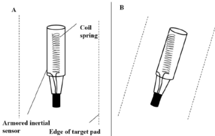
**Figure 2: Coupled inertial sensor inside the target pad: (A) – before the kick contact; (B) – after the kick contact (closed electronic circuit between the coil spring and the**
